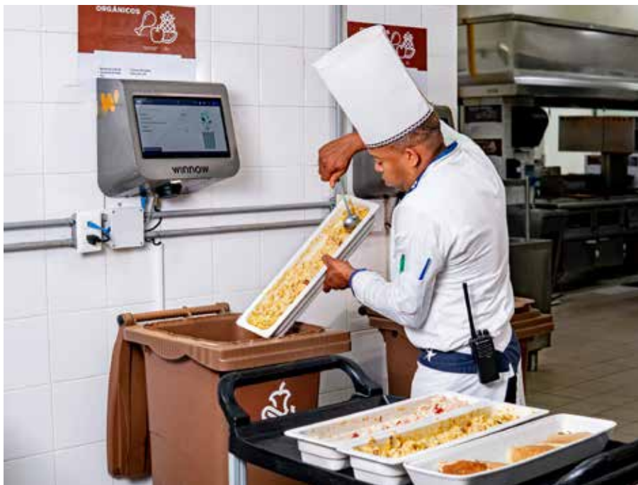
Winnow Vision uses AI and image recognition to track kitchen waste automatically—identifying items, assigning costs, and highlighting patterns that drive smarter purchasing and operations. The system captures everything from spoilage to uneaten meals, giving operators clear data to cut waste, save money and scale sustainability. Image courtesy of Winnow
